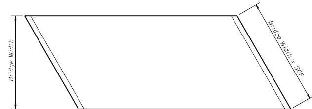
PLAN OF SUPERSTRUCTURE SLAB
